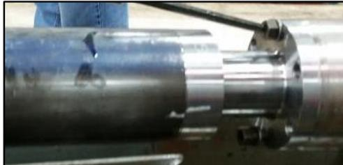
**Figure 14: Insert Top and Bottom Bolts**
