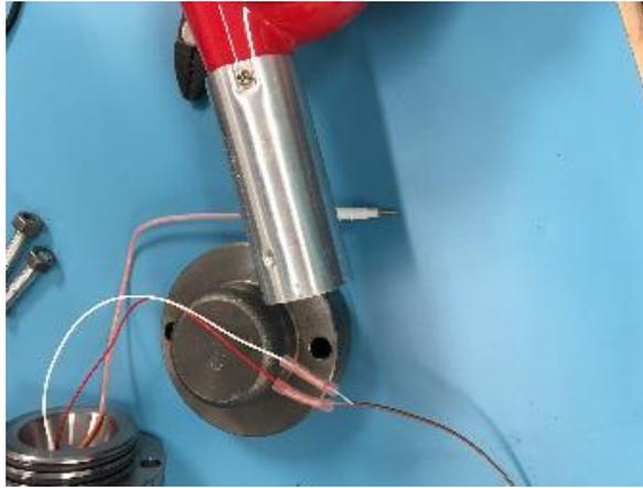
**Figure 6: Shrink Butt Splice Connections**
