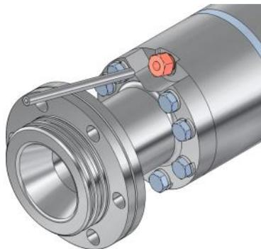
Insert tube into fitting until firmly seated against shoulder inside pressure head.
