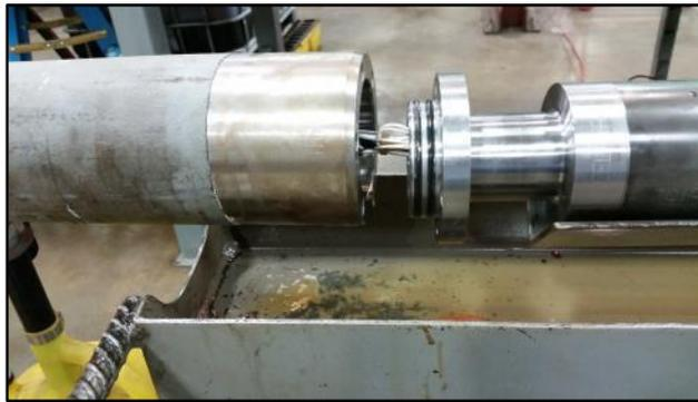
**Figure 13: Slide Wire Bundle into the Head of the Gauge**
