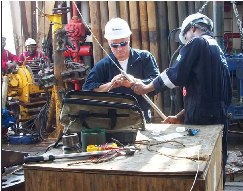
Figure 19. Pressure testing the cable head.
