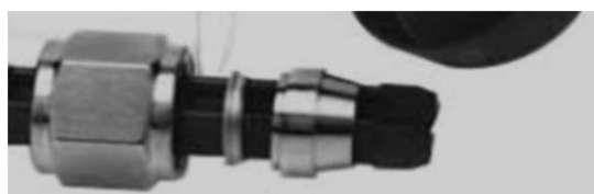
Figure 11. Correct orientation of ferrules as shown on Safety Changer.
